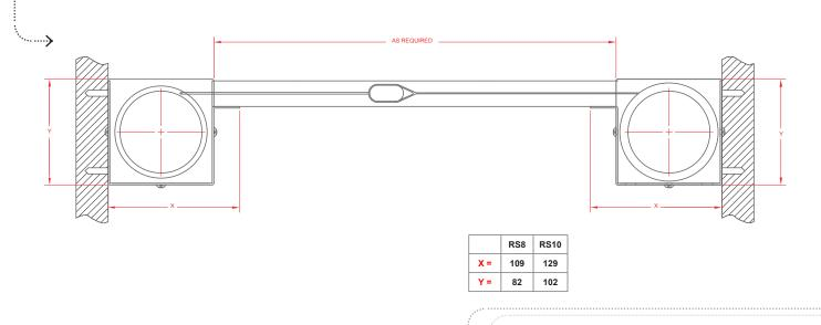
RECESS FIXING ARRANGEMENT
