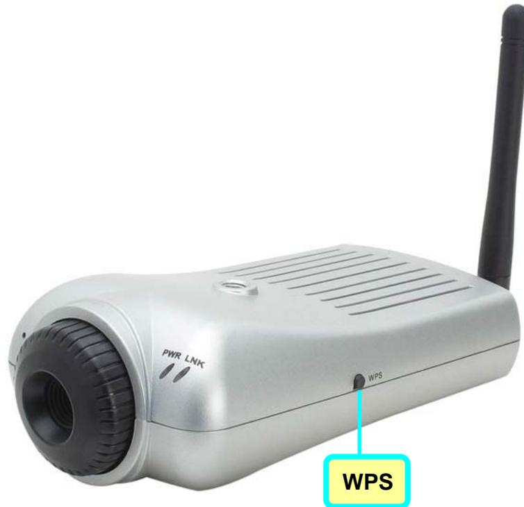
1. Before enable the WPS function, make sure the access point supports this function.
