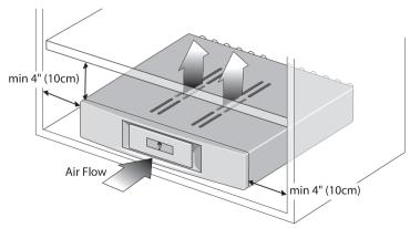
If the CHAKRA amplifier has inadequate ventilation and/or is played very enthusiastically for a period of time, its temperature may rise above the designated operating level and the affected channels will shut down until they have cooled sufficiently.
