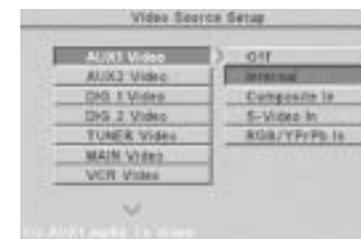
**COMPOSITE IN** - European version: When either the AUX 1 or AUX 2 source is selected, any video source connected to the CLASSIK Movie System Di's VCR SCART will be routed to the unit's TV SCART. US version: When either the AUX 1 or AUX 2 source is selected, any video source connected to the CLASSIK Movie System Di's CVBS IN will be routed to the unit's CVBS OUT.
