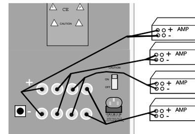
Quad-amped - 4 amplifiers. One drives the upper base unit, One drives the mid range unit. One drives tweeter unit and the final one drives the super tweeter.
