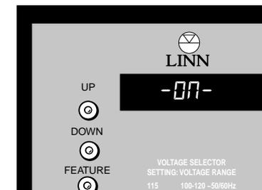
When the KOMRIS detect a signal, the display will change to "-ON-" and the bass system will start working.
