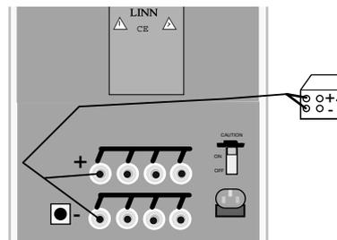
Connect the outputs of your power amplifier to the inputs in the KOMRI (see page 16 for more information). The speakers must be connected in phase (i.e red outlet on amplifier to red inlet on speaker)
