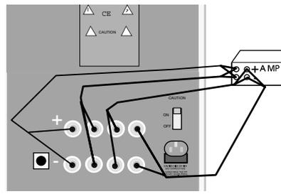
Quad wired - a single amp with customised common cables to drive all units.
