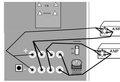
Bi-amp/Bi-wire - two amplifiers. One drives the upper base and mid range units. The other drives the tweeter and super tweeter units.
