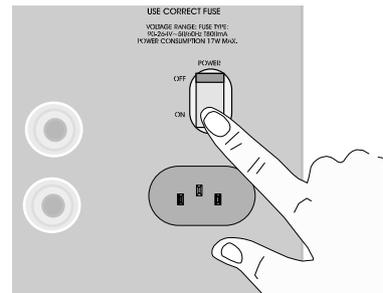
The KOMRI should always be switched off before connecting or disconnecting the power supply, as power surges which can damage the speaker may occur.
