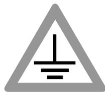
Always connect mains lead to an earthed power outlet.
