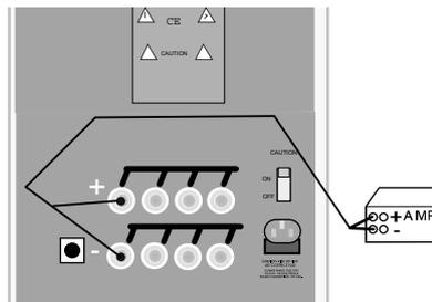
Single wire with link plate - a single cable from one amplifier drives each speaker.
