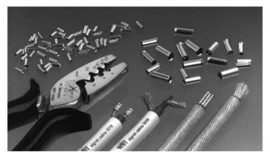
WBT offers a wide range of crimping accessories: gold-plated cable made of highly conductive electrolyte sleeves copper. E-Cu > 99.996% (in sizes from 0.5 to 16 mm<sup>2</sup>/22-5 AWG), sleeves made from fine silver (1.5 to 6 mm<sup>2</sup>/17-10 AWG), special crimping pliers for the above requirements and a complete crimping set for beginners. WBT-0403 crimping pliers/WBT-0411 crimping set.
